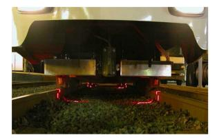
Fig.3: Alignment of Ultra sonic sensors
